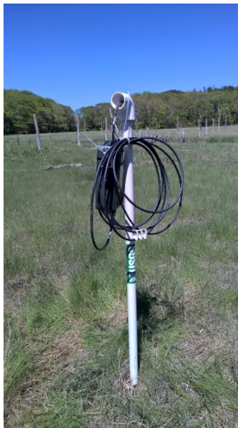
Figure 18 – Example of sensor equipped ground water quality in-situ monitoring site.
