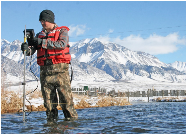
Figure 10 – Example of manual surface water quantity in-situ monitoring
