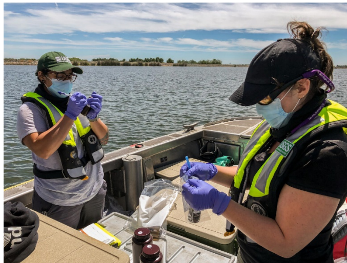
Figure 14 – Example of surface water quality sub-sampling for ex-situ analysis. USGS agents preparing samples (USGS)
