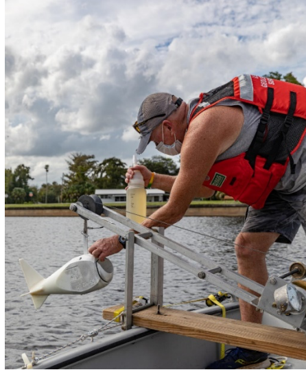
Figure 13 – Example of surface water quality sample for ex-situ analysis USGS technician loading a bottle into a DH-95 water-quality sampler (USGS)
