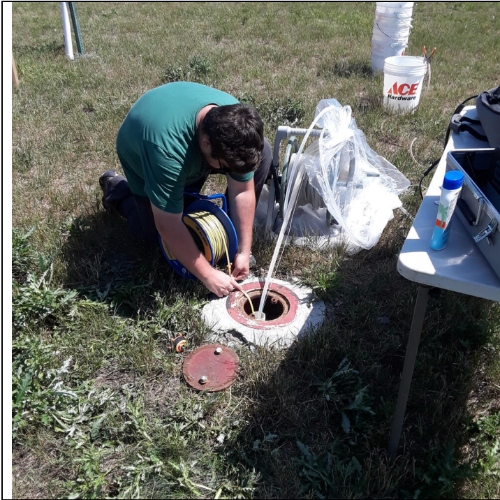
Groundwater-Level Measurement at Ellsworth Air Force Base | U.S. Geological Survey (usgs.gov)
