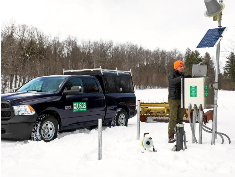
Figure 16 – Example of sensor equipped ground water quantity in-situ monitoring site.
