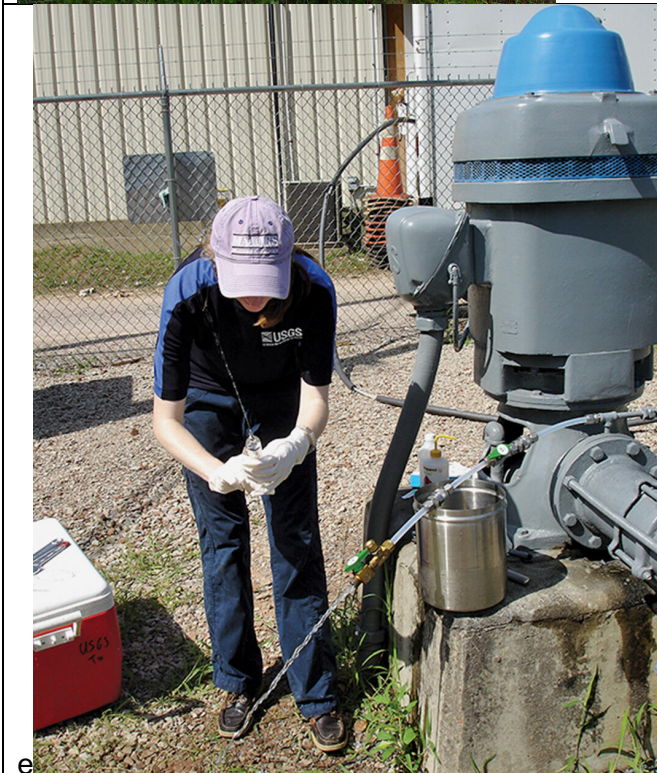
USGS employee sampling a public supply well for water quality analysis | U.S. Geological Survey
