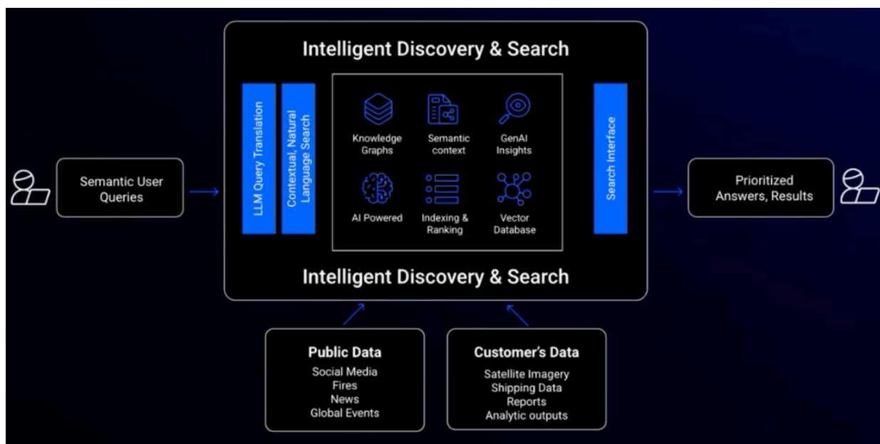
Figure 3 – D110 (Danti) - Logical Architecture Diagram
