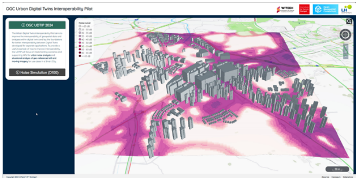
Figure A.62 – WiTech UDTIP Client Visualizing 3D City Model with Ground-Level Noise Data
