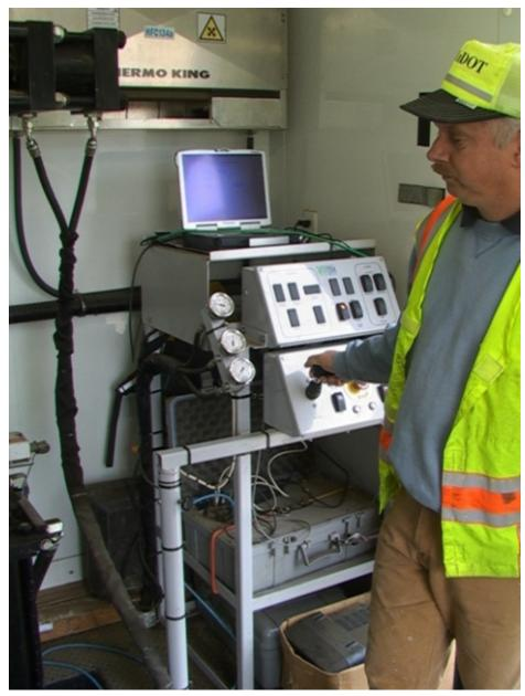
*Figure 26. Operator controlling the push rate as a CPT probe is advanced and data is automatically recorded by a data acquisition system. Photo courtesy of Minnesota Department of Transportation.*
