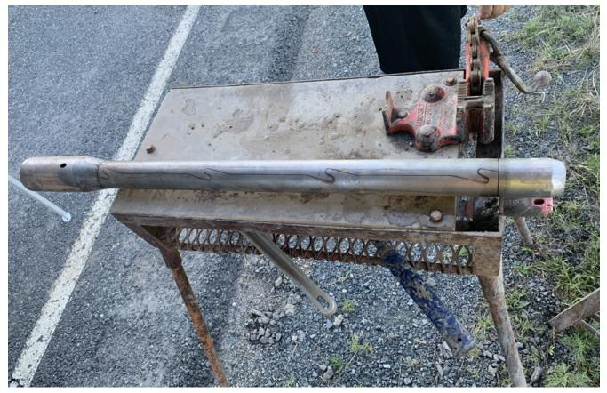
Figure 32. A SPT sampler rests on a work table, ready to be attached to the drill rods when the drill tooling is removed at the desired sample depth. Photo courtesy of Minnesota Department of Transportation.
