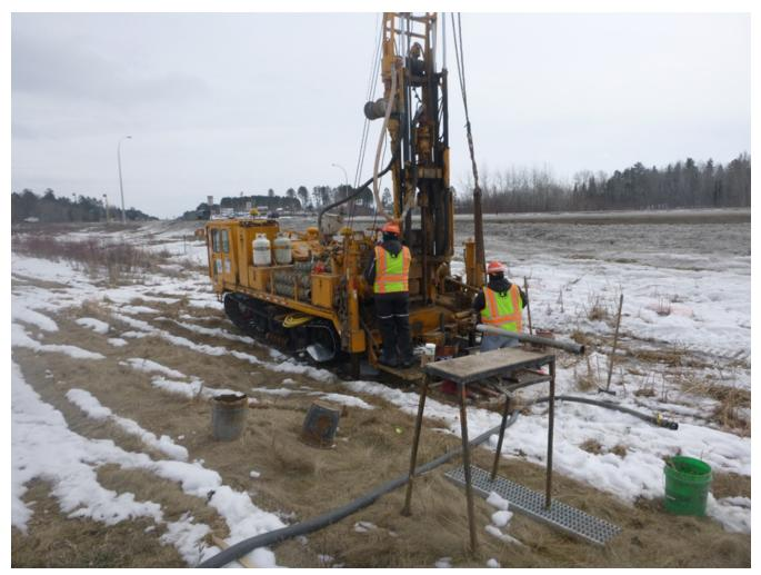
*Figure 31. A SPT drill rig on a project site; a work table with a SPT sampler is in the foreground. Photo courtesy of Minnesota Department of Transportation*
