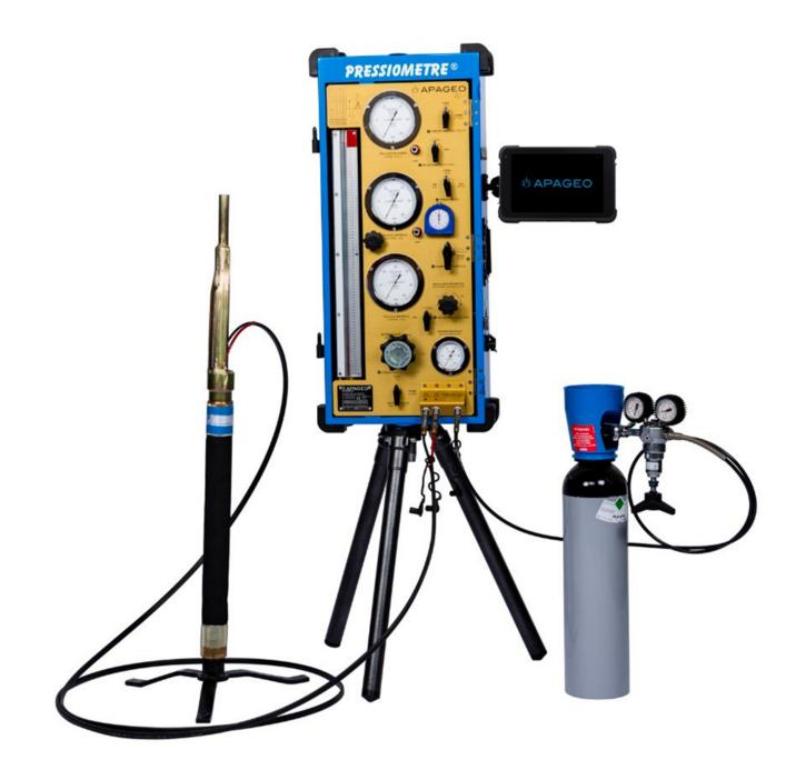
*Figure 35. Photograph of a pressuremeter set (extracted from https://www.apageo.com).*
