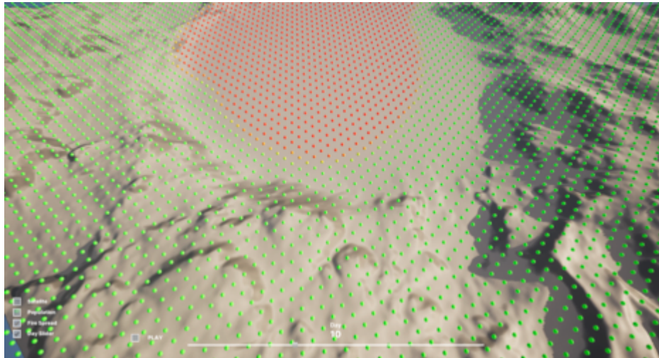
Figure 22 – This work-in-progress image shows (1) the creation of various terrain layers using DEM and soil, vegetation, and road network masks and (2) an example prototype of the Fire Fuel Indicator DRI overlaid on the 3D Site Twin.
