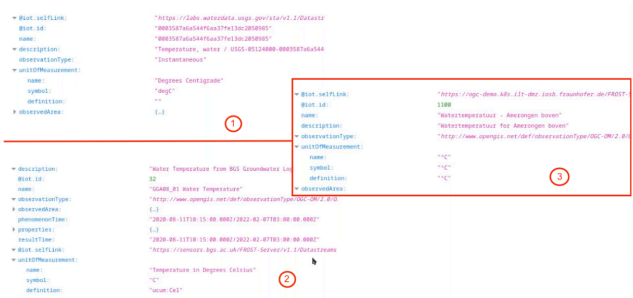
Figure 13 – Differences in Units of measure representation in a sample of SensorThings API instances
