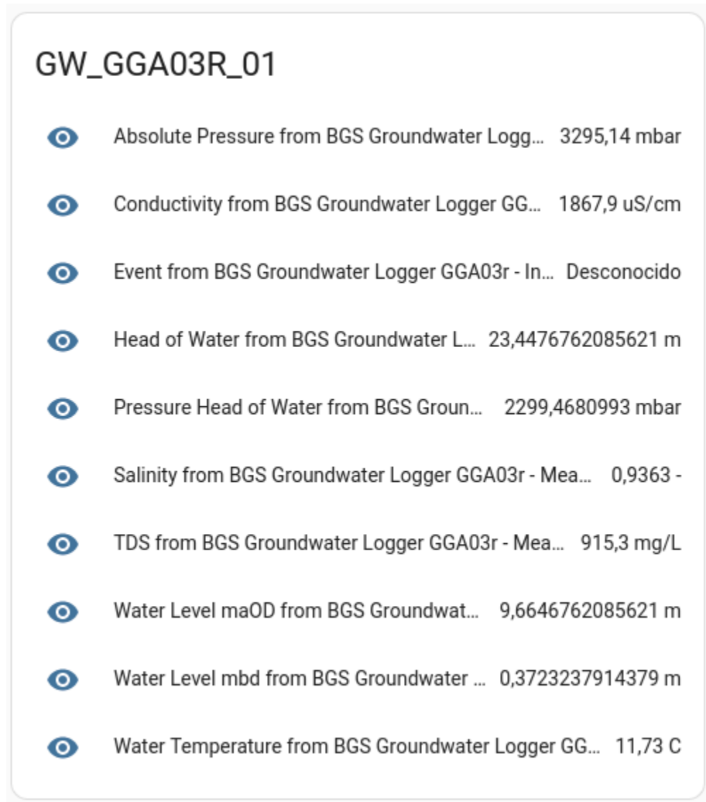
Figure 8 – Partial screenshot of a Home Assistant dashboard showing SensorThings observations from the British Geological Survey, from their FROST server.
