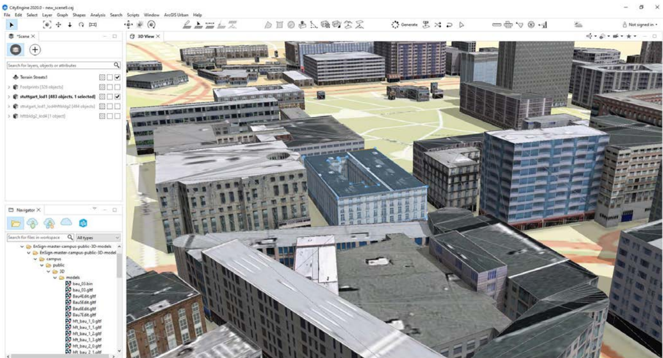
Figure 87. LOD-1 of 3D building models with generic textures displayed using ArcGIS CityEngine.
