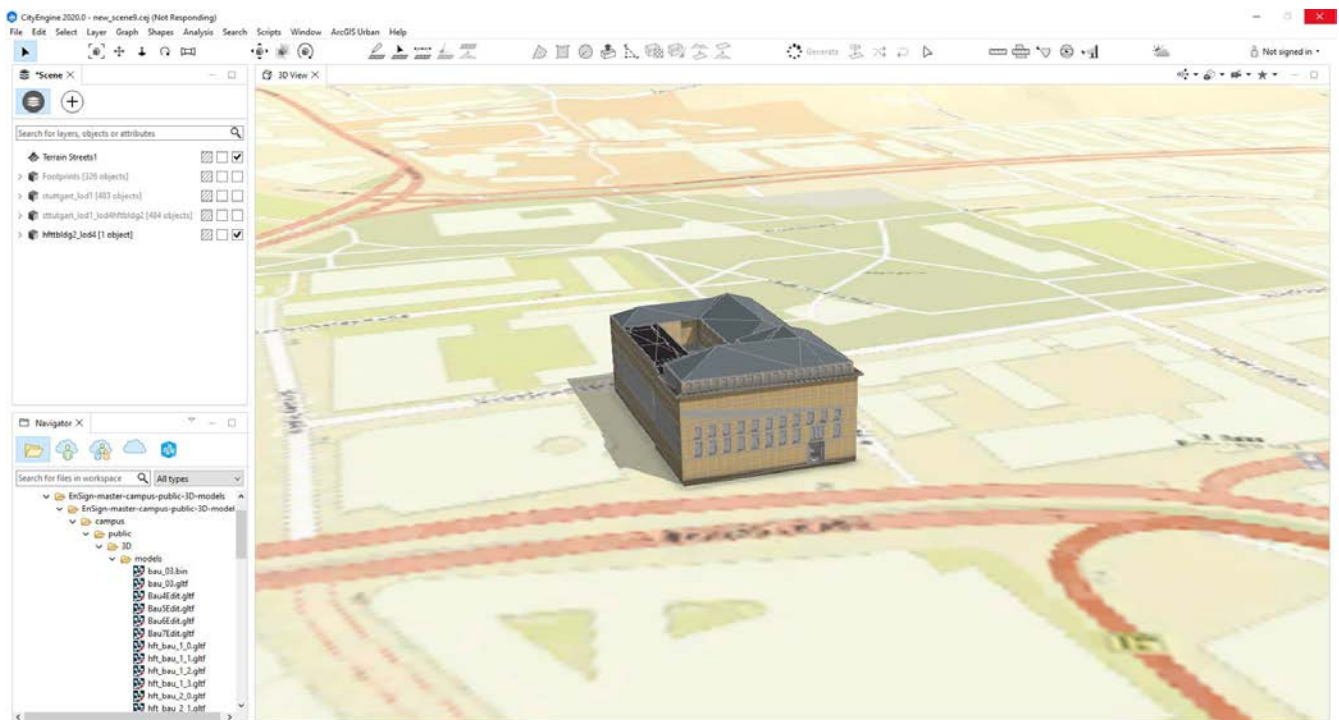
Figure 86. An example of a glTF model of HFT Stuttgart building imported into ArcGIS CityEngine.
