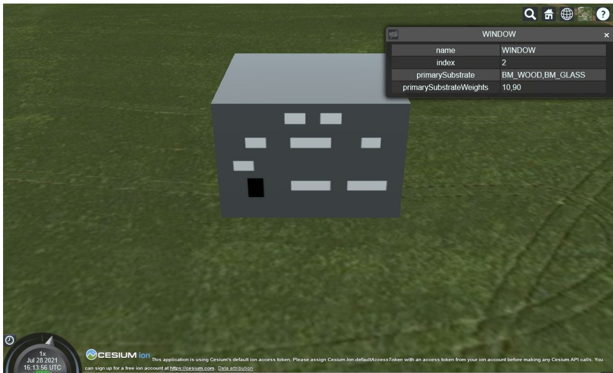
Figure 61. A simple model of a building rendered with a metadata texture.
