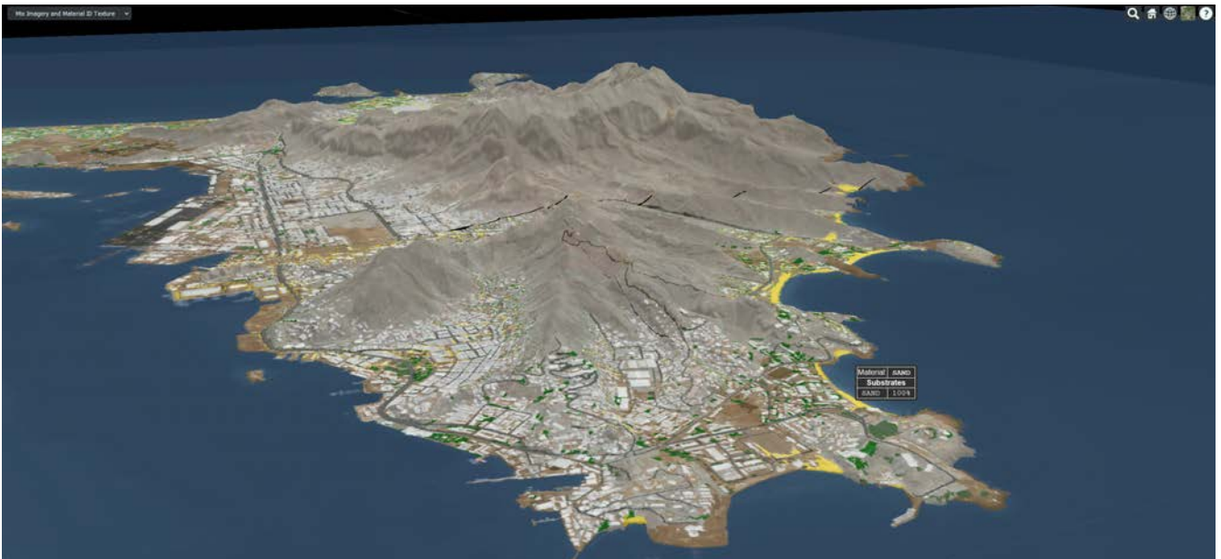
Figure 15. CesiumJS visualization of the per-terrain metadata from Aden, Yemen CDB. The metadata was overlaid on the satellite imagery of the terrain.
