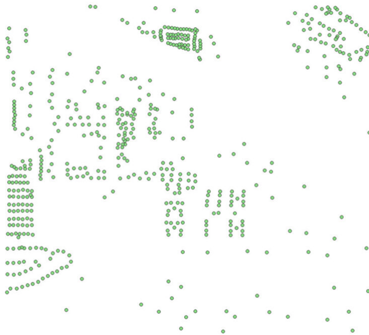
Figure 42. Mapbox Vector Tile of points positioning 3D buildings visualized in QGIS
