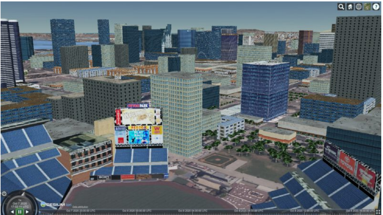
Figure 62. CesiumJS Client accessing San Diego CDB data as 3D Tiles from Ecere's GNOSIS Map Server (Petco Park)
