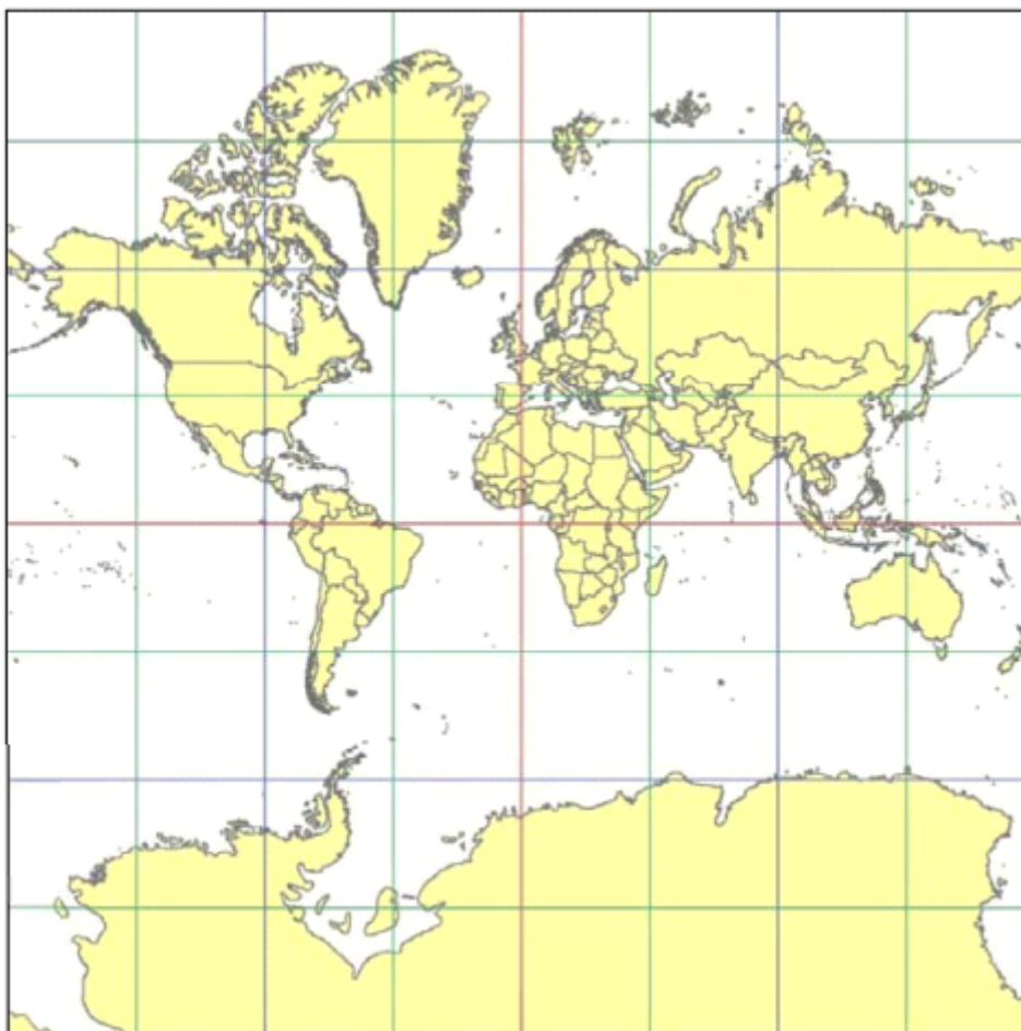
Figure D.3 – Tile Matrix Id 1 (red lines; 2x2 tiles) and 3 (blue lines; 8x8 tiles) of the WorldMercatorWGS84Quad TileMatrixSet (Source NGA)
