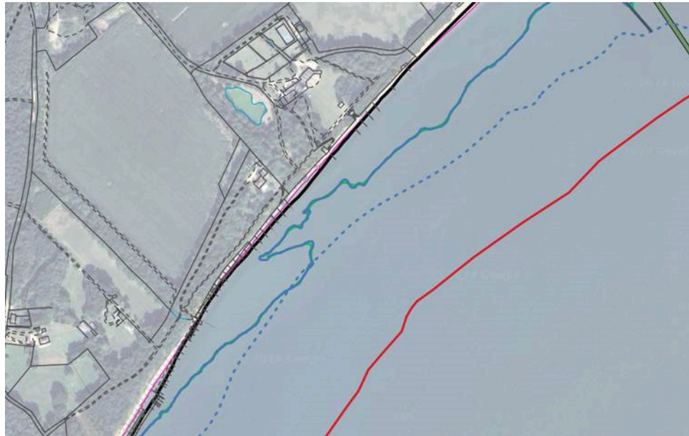
Calshot Bary: Red= S-57 LAT | Continuous Blue=OS MLWS (most products) | Dashed Blue =OS VML MLWS
