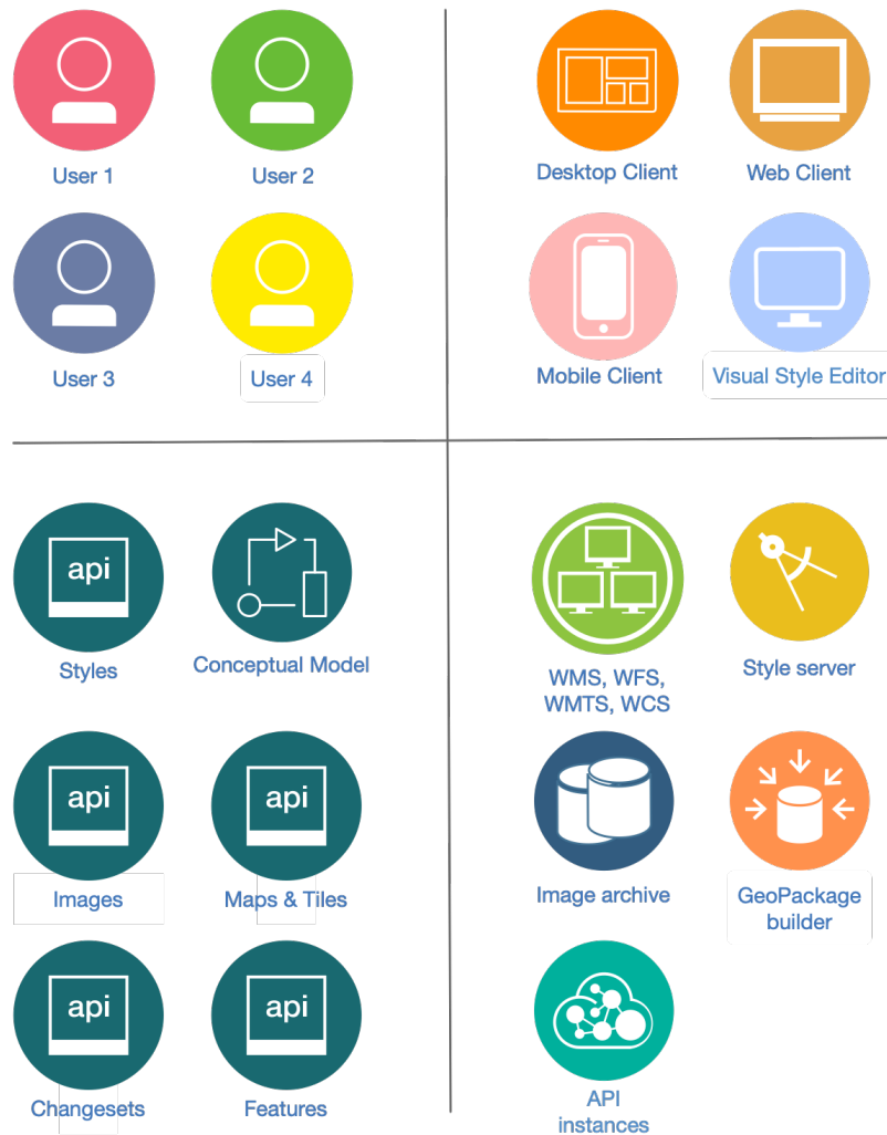
Figure 4. OPF components, with users in the upper left, client applications upper right, server technology lower right, and APIs lower left
