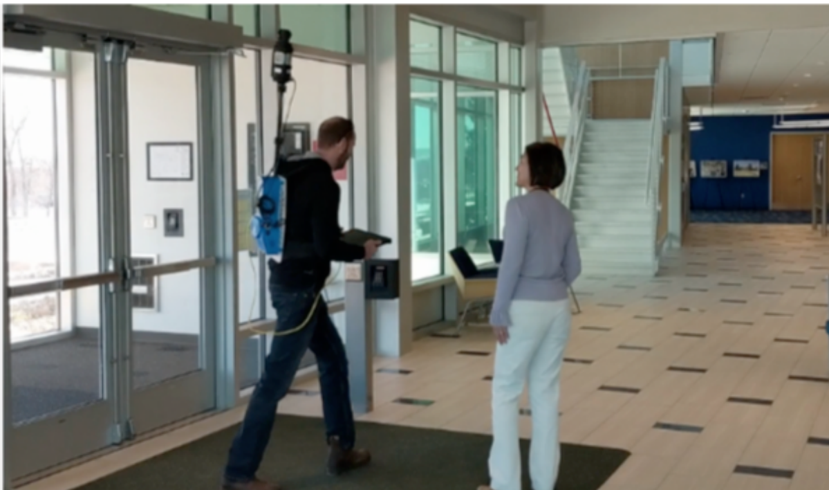
Figure 72. Mobile LiDAR Scanning Operation
