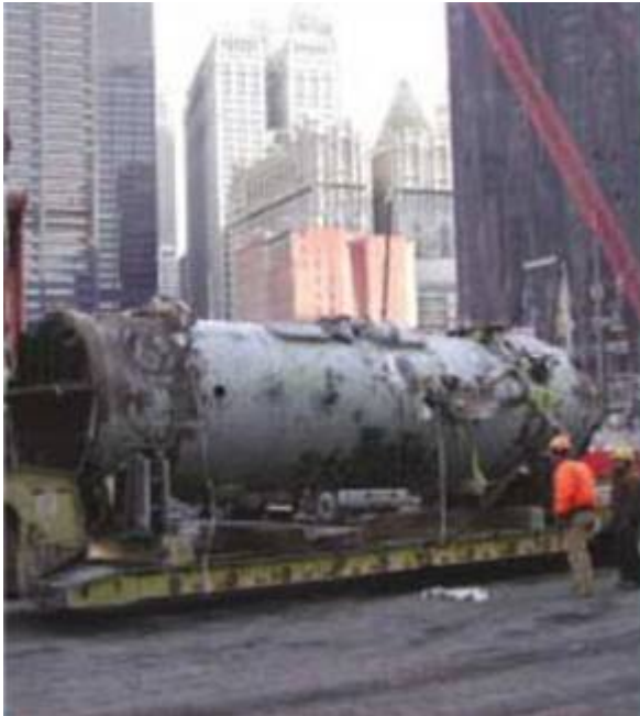
Figure 11. Unearthed Freon Tank from World Trade Center Site, Capacity 200,000 pounds ( https://www.osha.gov/Publications/WTC/dangerous_worksite.html )
