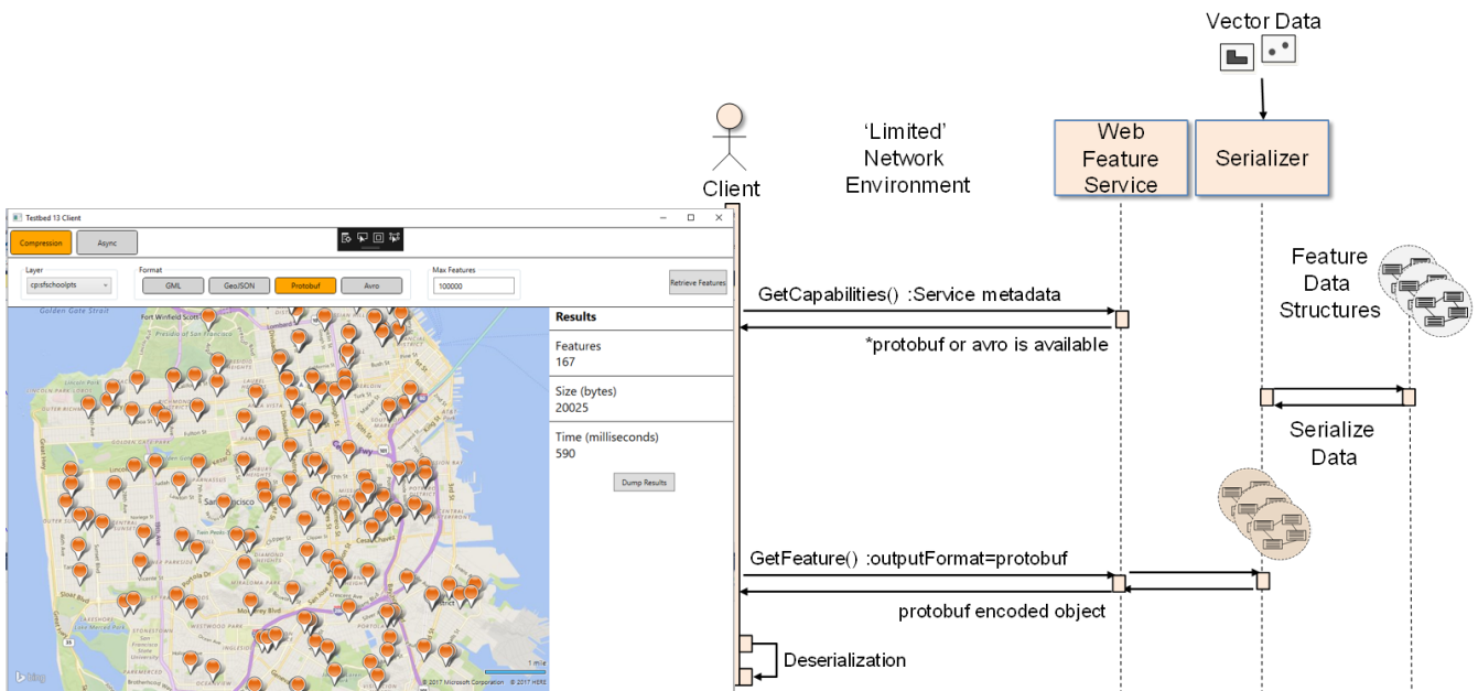
Figure 2. Sequence diagram for compression testing
